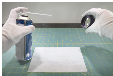
Abb. 7-1 Cleaning with compressed air
